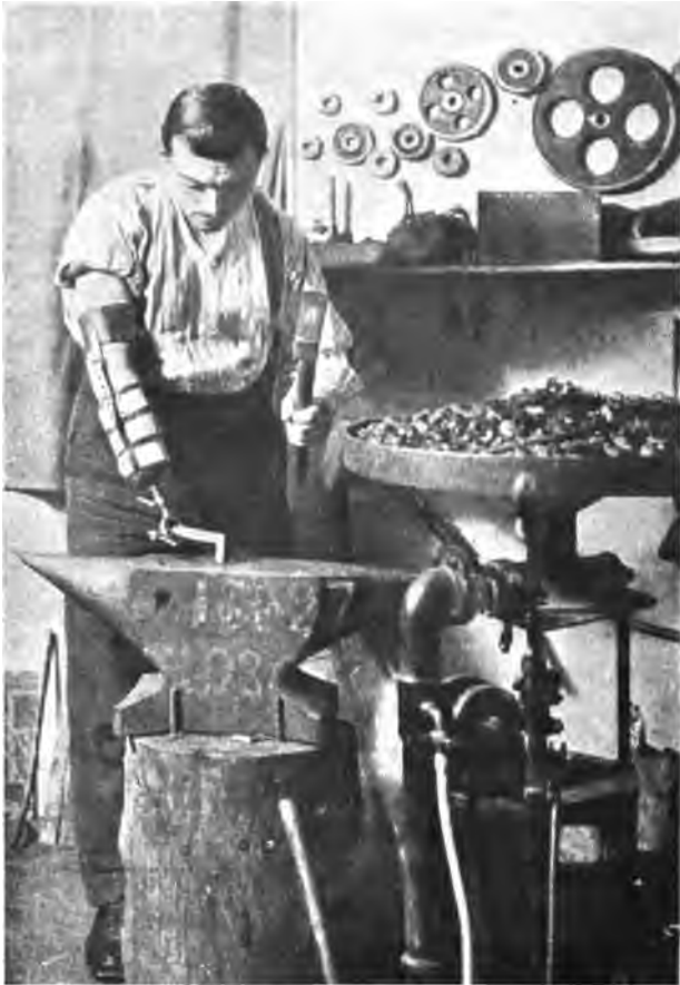
FIG. 130.—One-armed Mechanic making a Forging.
